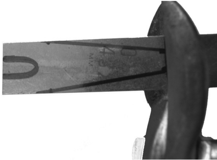
Spring stock marked for cutting a front spring.
