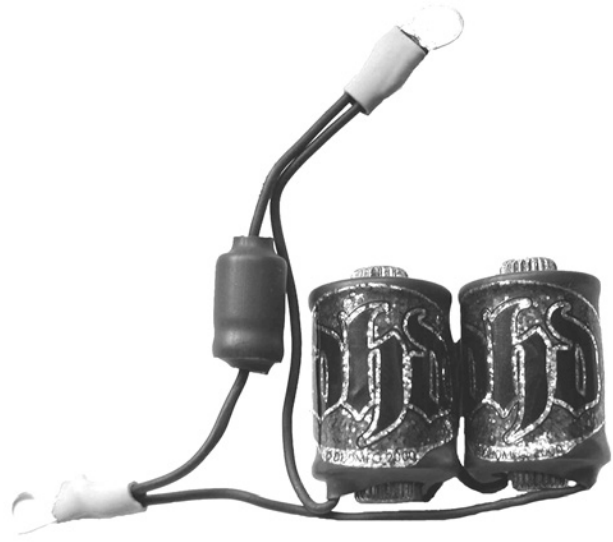
A properly insulated coil assembly.
